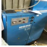
16044 Boge S 25 compressor 1995 max. working pressure: 8 bar rated motor power: 18,5 kW compressor: 400 Volt 50 Hz 3 ph cooling fan 2230/400 V 0,55 kW with emergency stop refrigeration dryer DS
