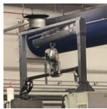
16556 Lifting hoist for anilox roller change (on R 700) 2007 for 3B size Roland 700 model
