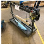
14909 Blanket wash roller rewinder 52-74-102 electric version
