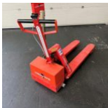
17912 Logitrans EHL 1000/3 electrical forklift Max. 1.000 kg.
