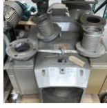
12290 Becker VTLF 500 vacuum pump 1998 Speed: 980 min Motor rating: 15 kW Inlet capacity: 500 m 3 /h Vacuum: 750 mbar
