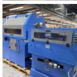
18134 Masuri VL-10 book splitting saw Bookblock feeder 1 splitting saw Turnover belt
