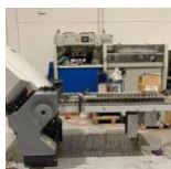
15295 Heidelberg TH 66/8 2nd folding station 8 buckles Anti-noise hoods
