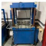
16601 Deal II strapping machine Double unit strapping, turner table to make the cross Siemens electronic program Strap width: 5 – 9 mm Capacity: with single strapping up to 35 packets per minute With double strapping up to 20 packets per minute
