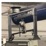
16556 Lifting hoist for anilox roller change (on R 700) for 3B size Roland 700 model
