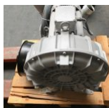
16157 G. Denver Rietschle SAP 530 side channel compressor pump (50/60 Hz) --) 590/710 m³/hour 5,5/6,5 kW/ 2900/3450/min 75/79 dB(A)
