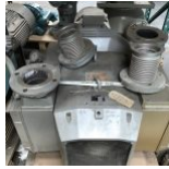
12290 Becker VTLF 500 vacuum pump Speed: 980 min Motor rating: 15 kW Inlet capacity: 500 m 3 /h Vacuum: 750 mbar
