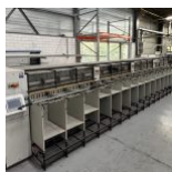
18049 Theisen & Bonitz Flex B316 SP+TB B304 QSM fully automated sheet collator with stich fold three knife trimmer
