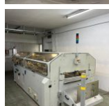
17294 Kolbus UKV 400 device for folded-in covers To be used as single machine or inline coupling with Kolbus cover feeder model NA401 Co-pilot with touch screen Automatic format settings Scoring device Folding-in zone Delivery tray
