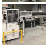
18143 Meccanotecnica Fido book block feeder For the automatic feeding of untrimmed, sewn, unglued, glued or perfect bound book blocks Equipped with feeding conveyer from the right
