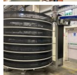
18166 Ambaflex 50 mt drytower 50 meter belts Entrance from the left under Exit to the right
