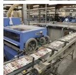
18214 Muller Martini 3502 splitting saw with 3506 turn-over belt By pass conveyer Infeed magazine Booksplitter 3502 Turn-over belt 3506
