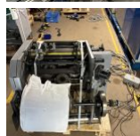
18218 Muller Martini Gauzing/Mull/Lining station To suit Muller Martini Acoro perfect binding line Equipped with: Motorised centring of lining strip (lateral adjustment) Quick Change Table Edge Cutting Device Trim Exhaust
